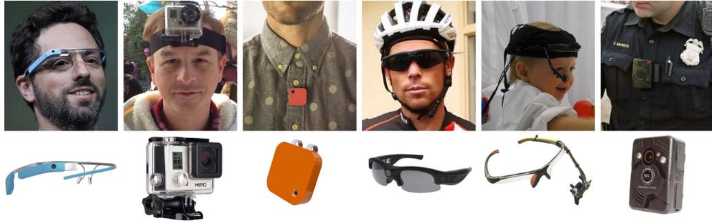
Figure 1.1: *Examples of different first-person camera devices.* From left to right: smart-glasses (e.g. *Google Glass*), compact outdoor cameras (e.g. *GoPro*), life-logging cameras (e.g. *Narrative Clip*), video glasses (e.g. *iVUE*), head-mounted eye tracking systems (e.g. *Positive Science*), and police body cameras (e.g. *PatrolEyes*).
